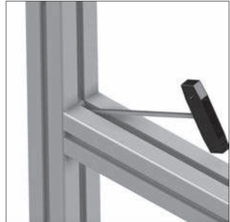
Install power-lock connector with button head screw on profile end, then undo the screw slightly so that the connector can be slid easily into the profile groove of the 2nd profile. Make sure that the inclined setscrew does not protrude on the outside. Tighten setscrew M8 using hexagon screwdriver SW4. Recommended tightening torque approx. 12 Nm
