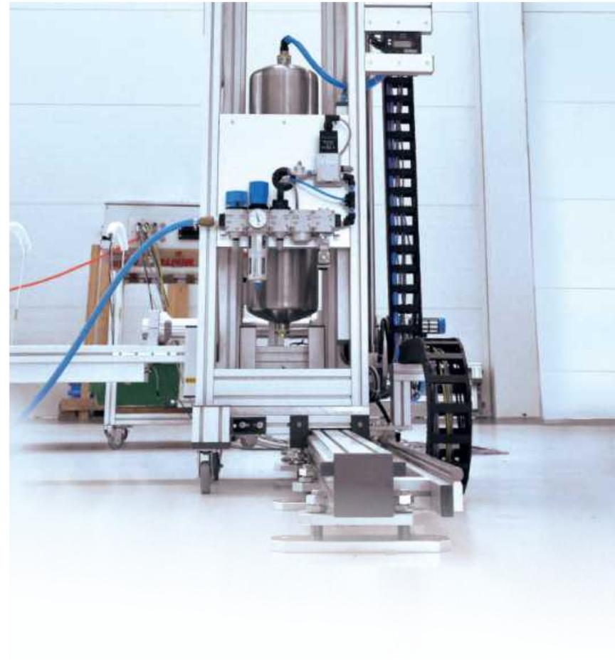
*The task of the system is to shoot the ice balls at the modules with a defined speed to check their strength. The ice balls can be shot from variable positions by means of carriages.*
